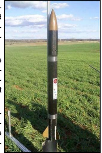
The finished rocket on the launch rail at the competition. Upon completion, it measured approximately 5ft tall and had a mass of 3 kg.
