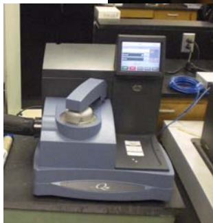
The Differential Scanning Calorimeter at CSU, used to determine the amount of heat required to increase the temperature of a sample.
