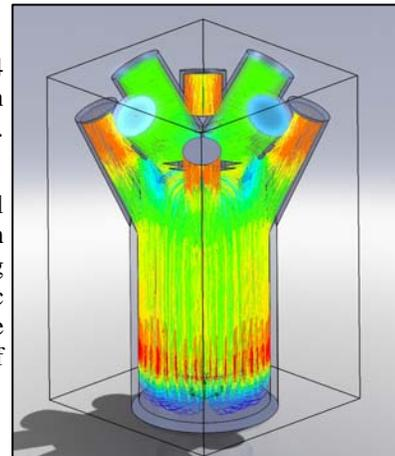
A Computational Fluid Dynamics Model Showing a Velocity Profile of the SMSR's Core. Red Lines Indicate Areas of Faster Flow and Blue Lines Indicate Areas of Slower Flow.
