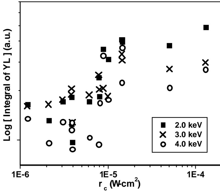
Figure 3. Integral of yellow luminescence as a function of contact resistance. There is a significant statistical correlation between the defect emission and increasing contact resistance. The trend is strongest at 2.0 and 3.0 keV
