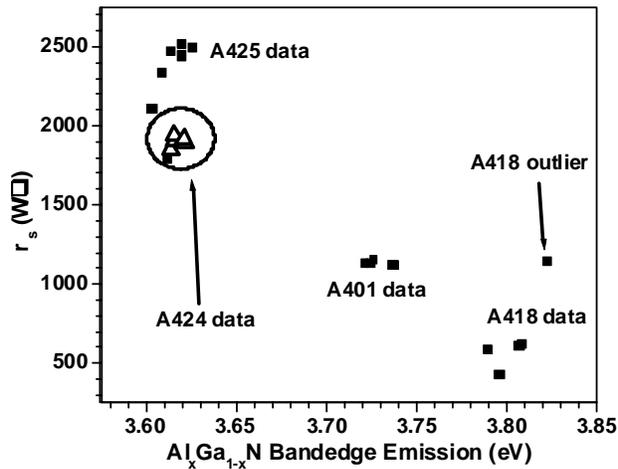
Figure 4. Sheet resistance compared to AlGa<sub>x</sub>N Bandedge. Note the uncharacteristically high sheet resistance on the outlier on A418
