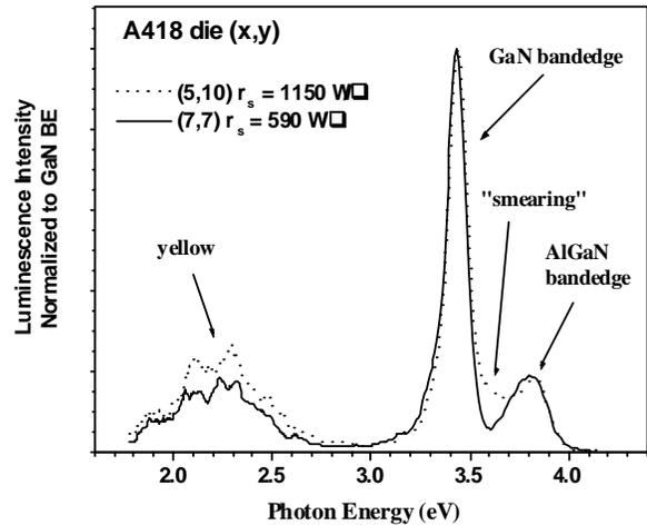
Figure 5. Spectra showing difference between good and bad sheet resistance on A418. On the die with high sheet resistance the AlGa<sub>x</sub>N Bandedge is smeared
