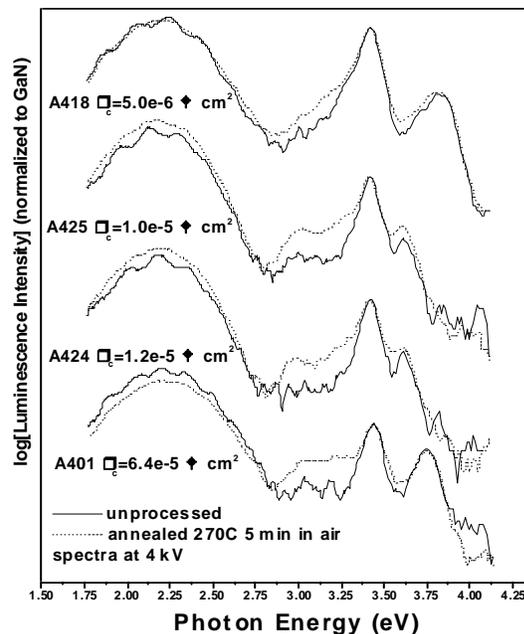
**Figure 2.** LEEN spectra at 4.0 kV of samples showing effect of air anneal on defect luminescence at 3.10 eV.
