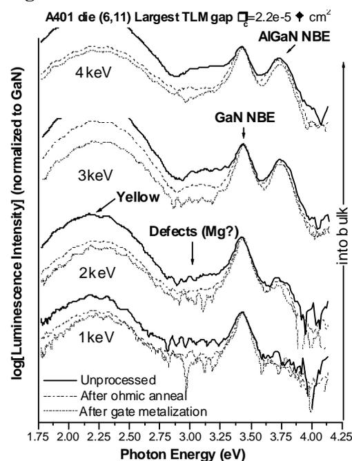
**Figure 1.** LEEN spectra of HEMT layer after various processing steps
