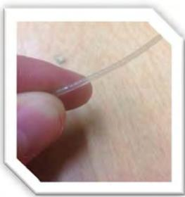
**Figure 2.** Manufactured SMP filament
