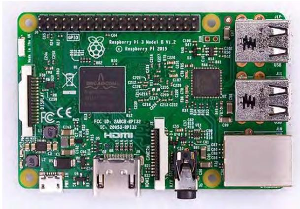
**Figure 1.** Raspberry Pi 3.0 Model B
