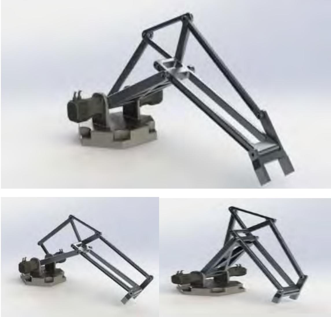
**Figure 2.** CAD Model of a Two Degree of Freedom Robot
