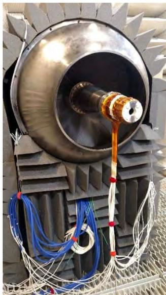
Figure 2. LAFPA setup on nozzle with co-flow
