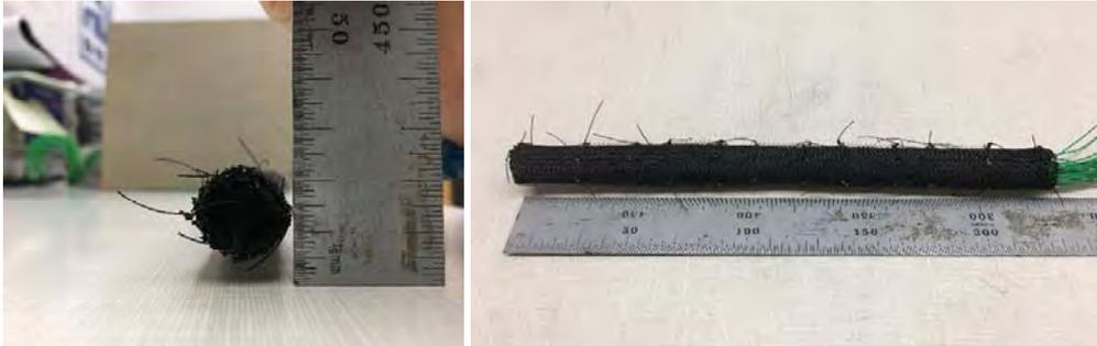
**Figure 3.** Version 2: front view at minimum diameter 1.8cm (left), and total length 23cm (right)
