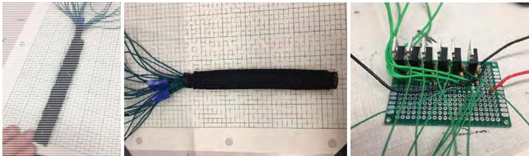
**Figure 2.** Mini-worm Version 1. Single mesh (left), double mesh (center), circuit board (right)
