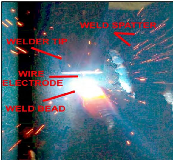
Figure 1. (Left) Parts of a weld.
