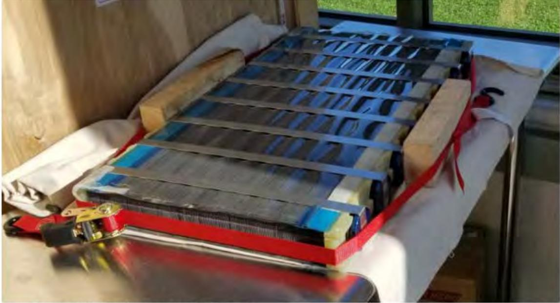
Figure 3 (above). One fuel cell stack removed.
