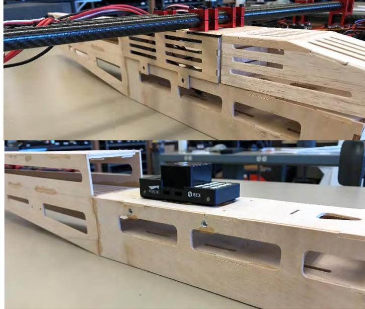
**Figure 3.** The wing mount gives easy access to the Pixhawk autopilot.
