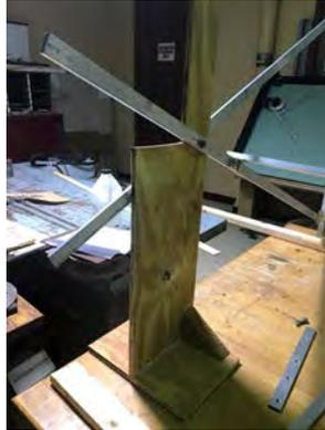
The base serves as an aid to rotate the lens frame in order to obtain the maximum solar energy by keeping the energy at the lenses focal point. Since the earth appears to rise from the east and sets in the west, we have implemented solar panels to direct the motor to rotate the base either clockwise or counter-clockwise through a shaft, 3 ½ " and 4" sprocket and chain pulley system using sprockets and bike chains. This rotation will follow the solar panels direction as the sun rises and sets.
