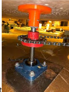
Center shaft with sprocket
