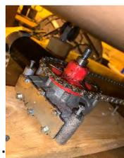
Motor and shaft with sprocket:
