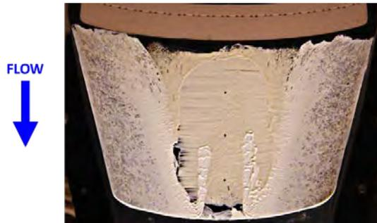
**Figure 3.** OFV of Separated Region at Mach 0.84.
