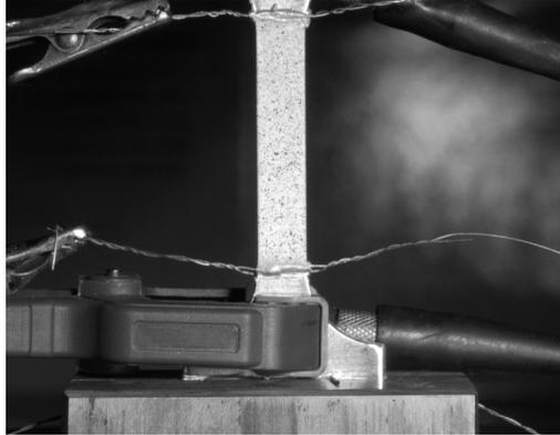
*Figure 1 - Inconel 718 specimen under tensile loading with AE, DIC, and ER NDE techniques involved*
