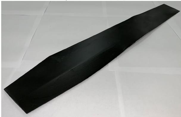
Figure 3. An example of a 85.3% scaled MSH rotor blade manufactured at OSU
