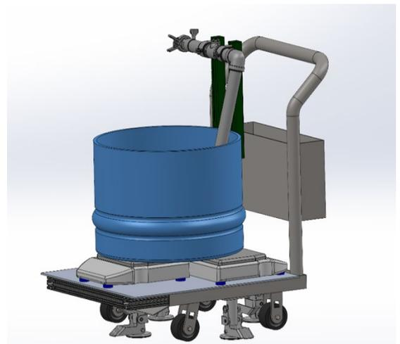
Figure 1: Flow Calibration Cart CAD Model
