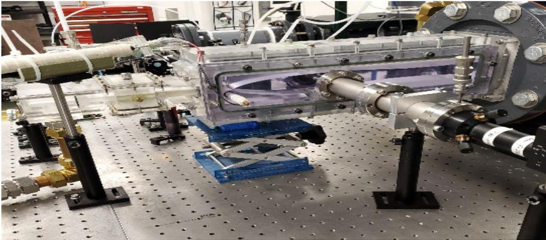
**Figure 1.** Unheated nonequilibrium flow supersonic wind tunnel (Mach 5) used for laser diagnostic measurements of excited species generated in the plasma sustained in the plenum or in the throat [1].
