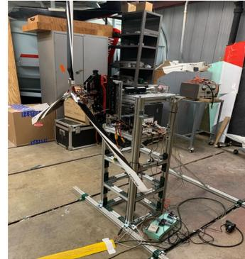
Figure 2. Isolated rotor test stand with symmetric airfoil rotor blades
