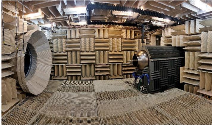
Figure 1: Anechoic jet chamber at Ohio State's Aerospace Research Center
