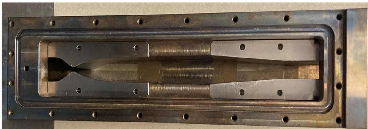
**Figure 5.** Mach 4 nozzle, supersonic flow diagnostic section, and supersonic diffuser. Flow direction is left to right.
