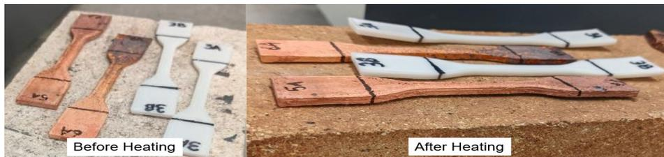
Figure 3: Samples Before and After Heating for 30 min at 80 °C
