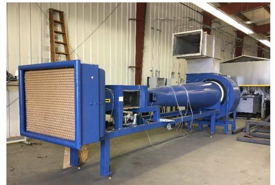
Figure 2: Open-type wind tunnel to be used for project.
