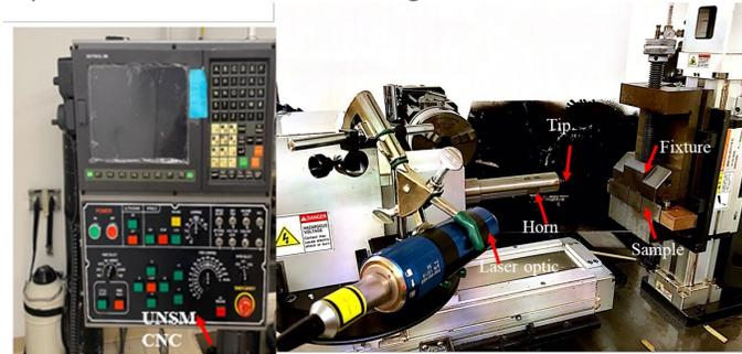
*Figure 2 - The University of Akron's LA-UNSM machine with accompanying CNC panel*
