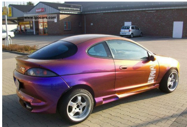
Ford Puma with interference pigment paint [Car photo: source ]
