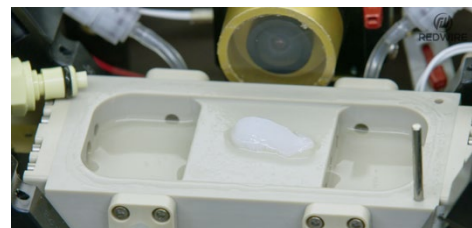
Figure 1: 3D printed knee meniscus by Redwire.
